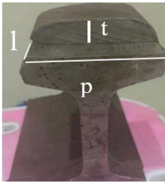
Figure 13. Cutting Dimensions of R.54 Rail Sample Source: Personal Documentation
